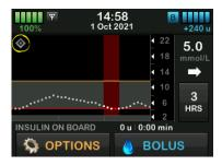
When Basal-IQ technology is enabled and active (i.e. insulin delivery has been suspended), the lower half of the diamond icon will be red. In addition to the diamond icon, other screen visuals indicate that insulin has been suspended, including:
