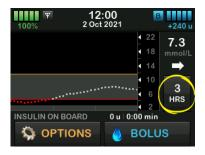
6 Hour Trend Graph shows you your current glucose reading along with the last 6 hours of sensor glucose readings.
