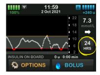
1 Hour Trend Graph shows you your current glucose reading along with the last 1 hour of sensor glucose readings.
