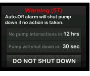
✓ The warning clears and the pump returns to normal operation.
