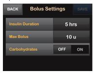
Using the onscreen keypad, enter the desired time for the duration of insulin action (2–8 hrs) and tap DONE.
