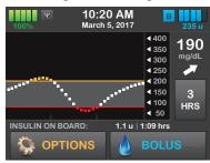
6 Hour Trend Graph shows you your current glucose reading along with the last 6 hours of sensor glucose readings.
