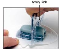
Transmitter with Safety Lock snapped in
