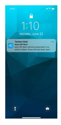
Unlock your smartphone and open or navigate to the Tandem Mobi mobile app. The Auto-Off Alarm timer will reset automatically once the Tandem Mobi mobile app is open.
