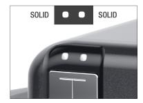
The pump LED status indicator will also indicate charge amount. When charging, the LED status indicator will display one pulsating light if the charge amount is less than 50%.
