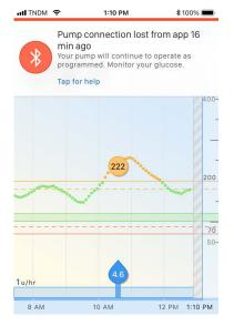
The *Notifications* screen will also display this alert, but you will not receive any new notifications on the Tandem Mobi mobile app until the pump reconnects.
