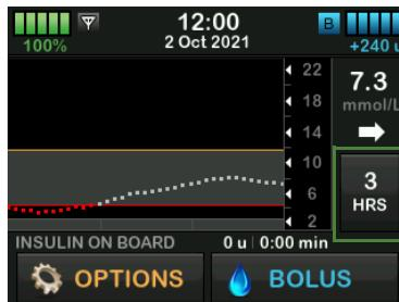
6 Hour Trend Graph shows you your current sensor glucose reading along with the last 6 hours of sensor glucose readings.
