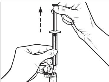
5. Make sure the needle is still in the fill port and release the plunger. Pressure will pull the plunger to its neutral position but it will NOT push any air back inside the cartridge.
