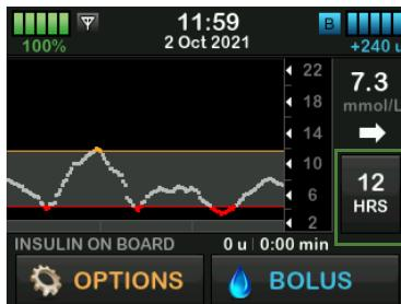
24 Hour Trend Graph shows you your current sensor glucose reading along with the last 24 hours of sensor glucose readings.
