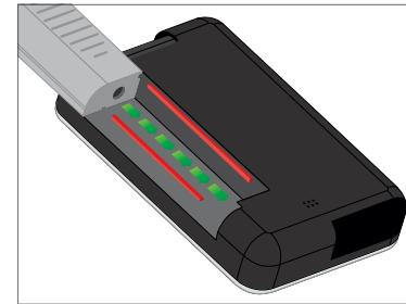
8. Push on the circular fill port next to the cartridge tubing to slide the
