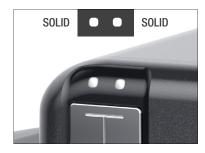
The pump status lights will also indicate charge amount. When charging, the pump status lights will display one pulsating light if the charge amount is less than 50%.
