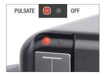
The pump continues to operate normally while charging. You do not need to disconnect from the pump while charging.
