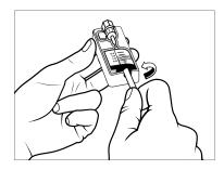
Press the release tab and pull the vial adapter forward to remove the cartridge from the set.
