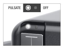
When the charge amount is above 50%, the pump status lights will display one solid white light and another pulsating white until fully charged. These lights will remain lit until fully charged.
