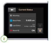
Your pump will display the name of the user's active profile, the current basal rate, the time and amount of the last bolus, and whether or not they are using Basal-IQ technology.
