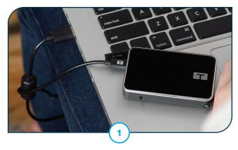
Plug the pump into the computer using the USB cable provided with the t:slim X2 pump
