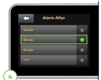
4 Select the button that corresponds with the time you would like the Resume Pump Alarm to display.
