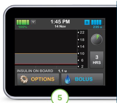
The pump will return to the Home screen with a CGM trend graph and sensor startup countdown symbol.
