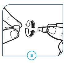
Connect the infusion set tubing to the cartridge.
