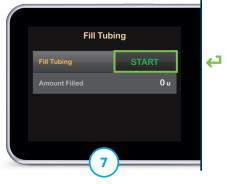
Hold the pump and tubing vertically and then tap **START.**
