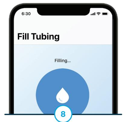
Release Pump button after three drops of insulin are seen at the end of the set.
