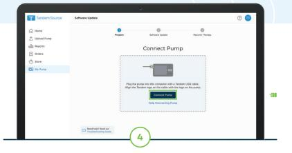
Connect the micro-USB end of the USB cable provided by Tandem Diabetes Care to the insulin pump and connect the other end to a USB port on the user's computer. Click **Connect Pump.**
