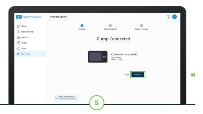
A Pump Connected screen will appear if the connection is successful. Confirm the pump serial number is accurate before clicking **Continue**.
