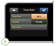
Tap **Duration**. Using the onscreen keypad enter desired length of time for Temp Rate. Tap to continue.
