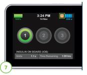
The Lock screen will appear with the orange T icon indicating a Temp Rate is active.
