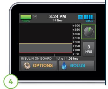
4 A symbol will appear on the Home screen to indicate the two-hour startup process has begun. During this time, the user will not receive sensor data or be able to use advanced features such as Basal-IQ technology.
