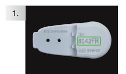
Locate the ID on the bottom of your transmitter before attaching it to a sensor.
