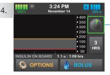
A screen will appear to indicate the two-hour startup process has begun. During this time, you will not receive sensor data or be able to use Basal-IQ technology. NOTE: The countdown symbol fills in overtime to show how much time is left before the system is ready to display current CGM reading.
